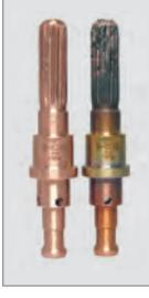
Electrodes – both new and worn, showing signs of possible moisture in the incoming gas. Excessive moisture will alter the characteristics of the plasma stream degrading performance. The use of a filter is recommended with some manufacturers advising air dryers.
